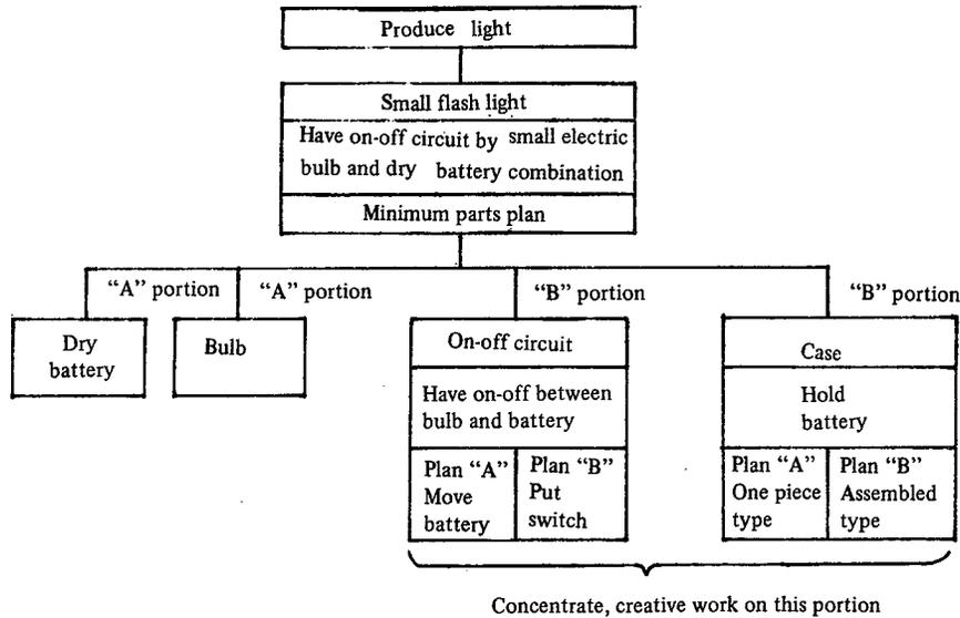
Fig. 4. FBS Block Diagram of Small Flash Light
