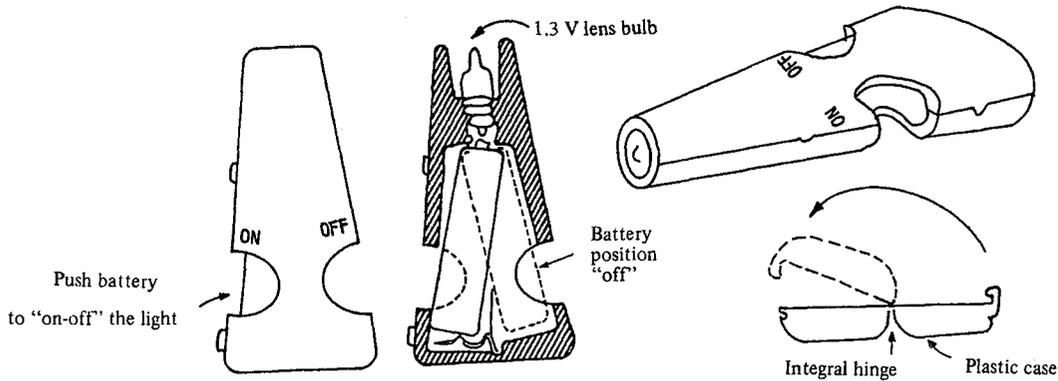
Fig. 5. Example of Small Flash Light Design.
